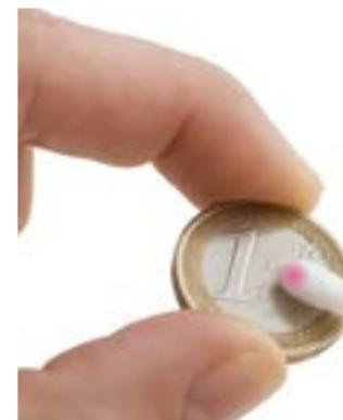
**Chemo Nickel Test™ (NT) and Chemo Cobalt Test™ (CoT)** are one-component solutions that enable easy detection of free nickel or cobalt in metallic objects.
